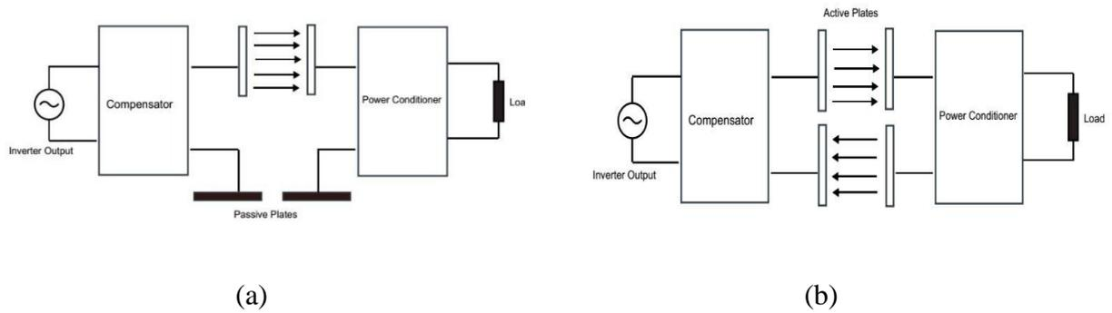
**Figure 4.** Unipolar demonstration coupling (a), Bipolar demonstration of capacitive coupling (b)
