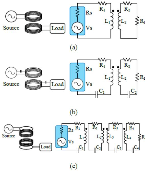
**Figure 2.** Topologies of (a) traditional IPT, (b) coupled magnetic resonance, (c) Strongly coupled magnetic resonance
