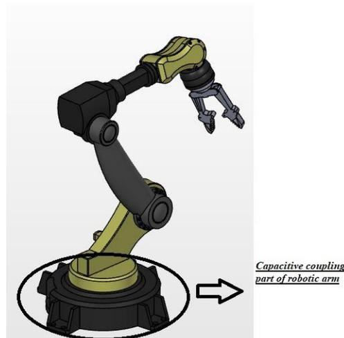
**Figure 5.** The capacitive coupling application with robotic arm
