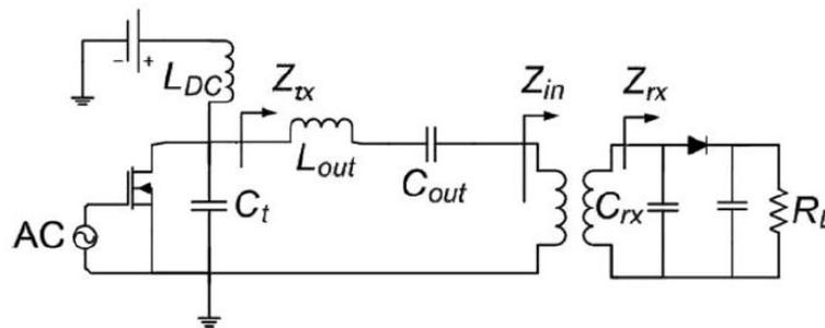
**Figure 3.** Class-E power amplifier circuit
