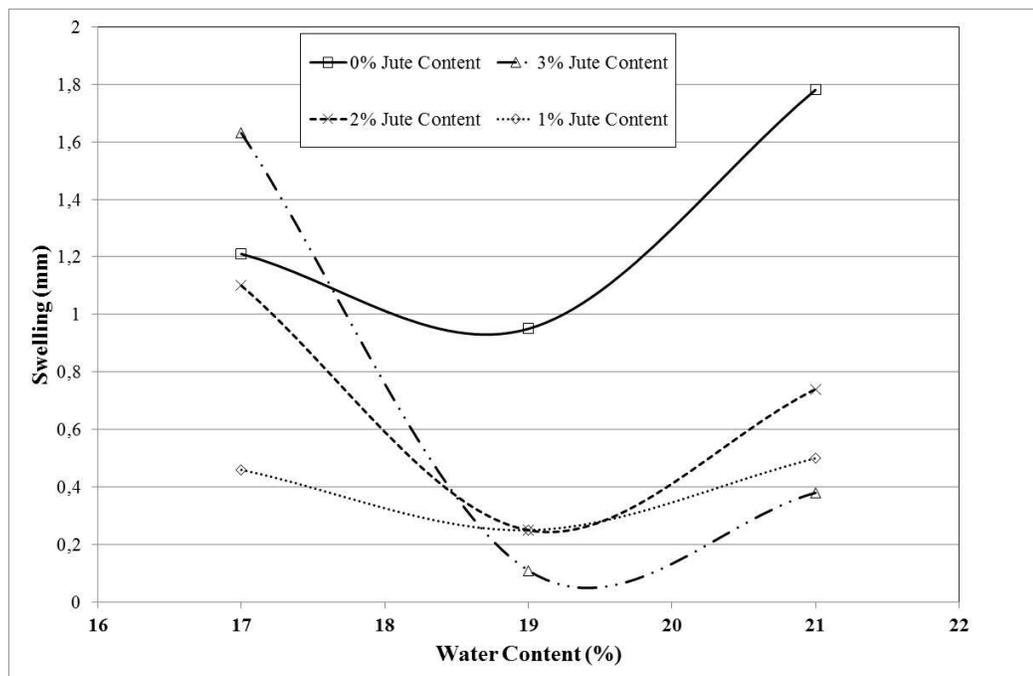
Figure 5. Water content-Swelling behavior of the specimens
