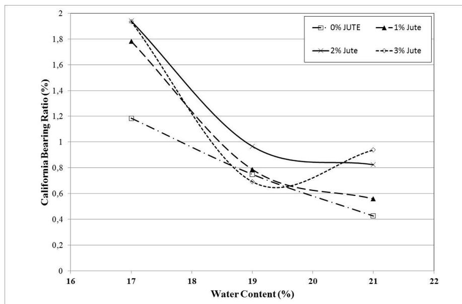
Figure 2. Water content-CBR behavior of the specimens.
