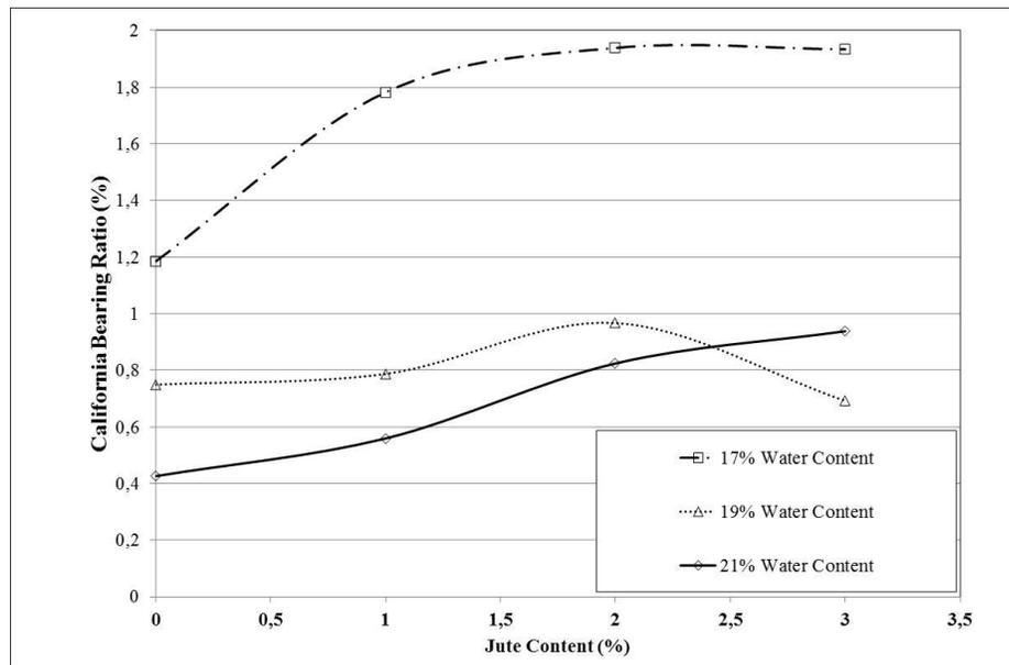
Figure 3. Jute content-CBR behavior of the specimens
