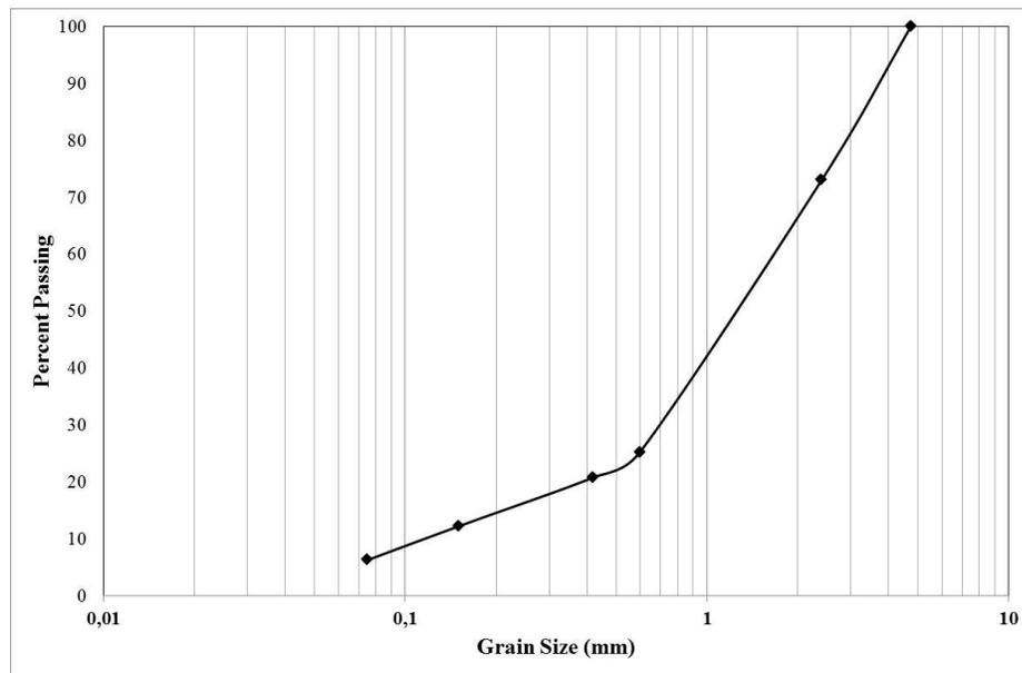
Figure 1. Size gradation curve of the soil
